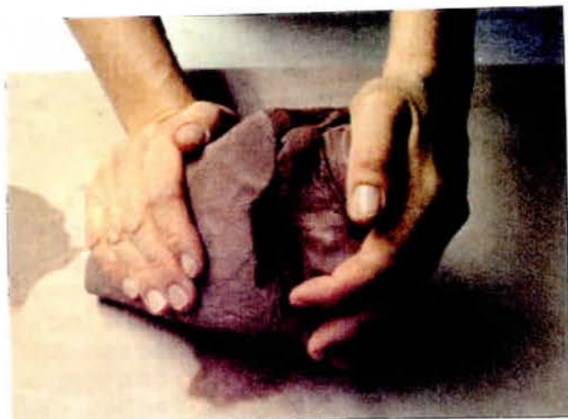
(fig. 1) Spiral wedging causes the clay to become cone shaped.
