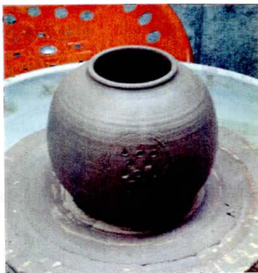
(fig. 10) Several small circles are cut to serve as a strainer for tea.
