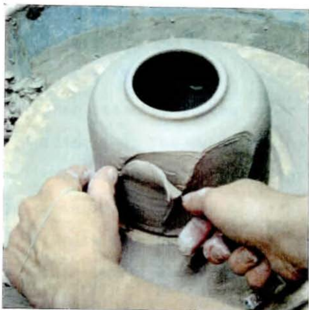
(fig. 13) The width and thickness of the faceted slice must be precise.
