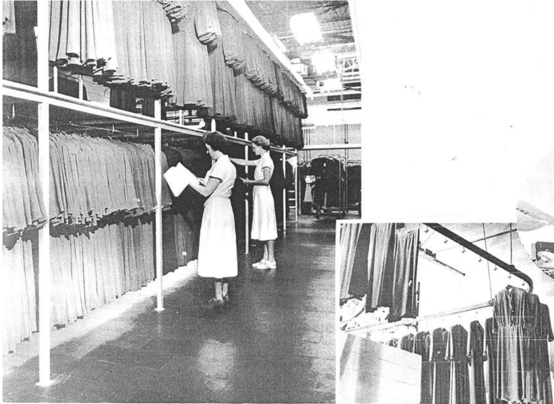
Figure 10. The “moving finger”; a new conveyer system that carries dresses from the ultra-modern pressing room to shipping area where they hang color by color in double – deck cabanas ready for delivery to 2,500 stores worldwide (c. 1940s) (The State Historical Society of Missouri Research Center-Kansas City, Nelly Don at Home Catalogs , folder 35).
