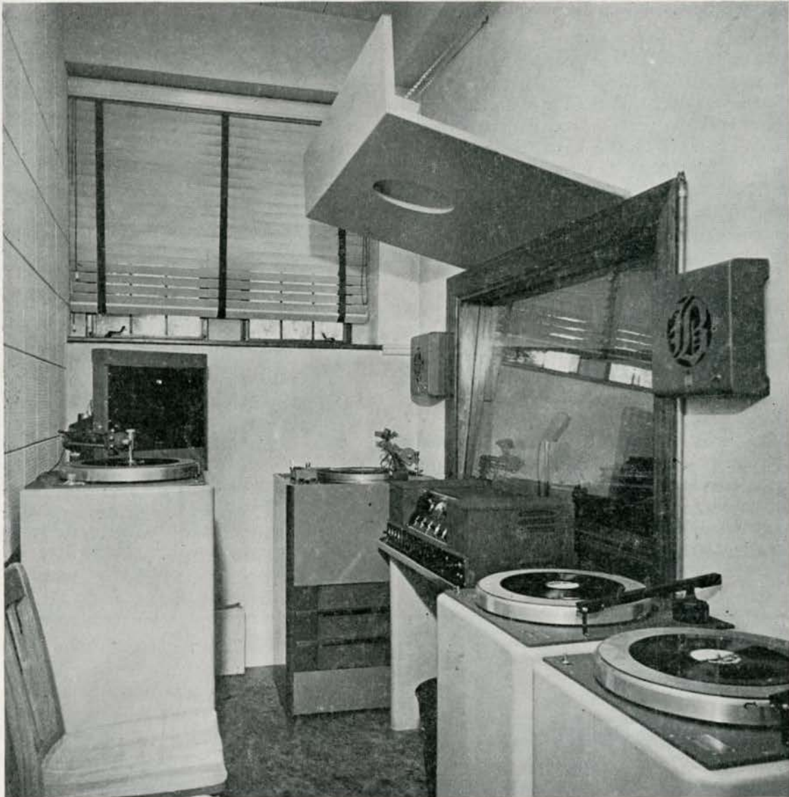
Lindenwood now has some of the most modern radio and recording equipment in American colleges today. This is a view of the soundproof control room of the Radio Studio in the Lillie P. Roemer Fine Arts Building, showing the control panel, mixing board, cutting tables, playback machines and the communication system to the broadcaster.
