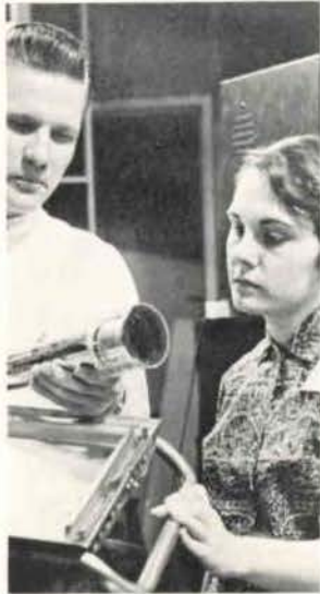
KETC engineer explains the camera's heart , the video tube—a small item worth more than $1000.
