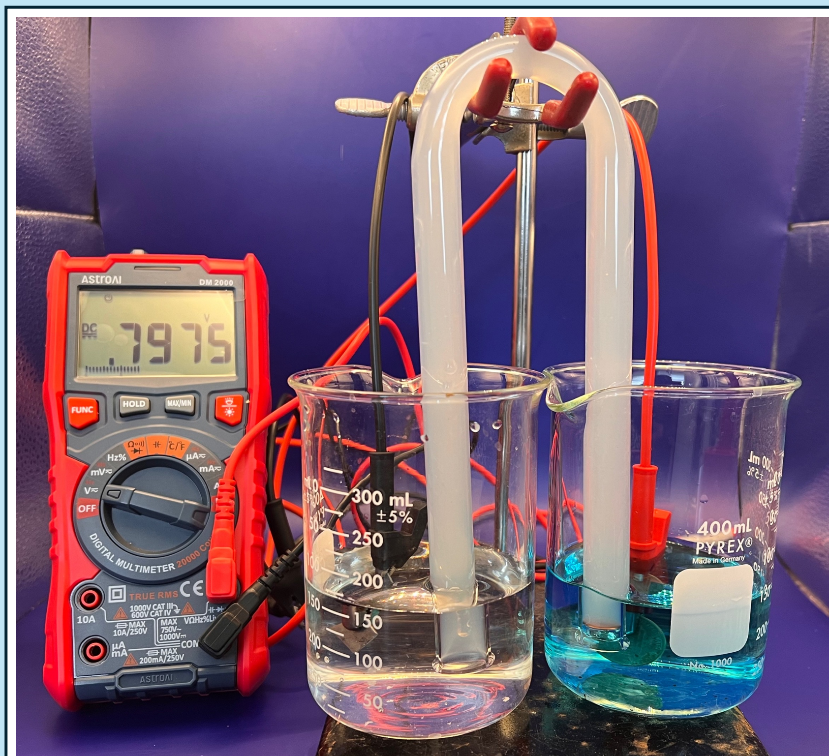
Electrochemical cell with \text{Cu(s)} \mid \text{Cu}^{2+} (.125 \text{ M}) \parallel \text{Zn}^{2+} (.1 \text{ M}) \mid \text{Zn(s)}
